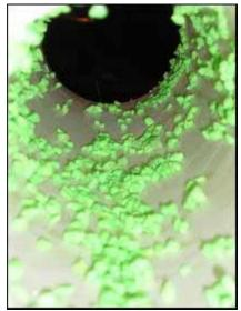
Figure 4.4 Low to moderately tuberculated pipe model
