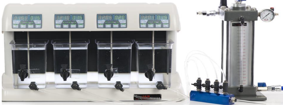
2L DAF Jars in place at a Platypus 4G Jar Tester, manifold and Saturator
