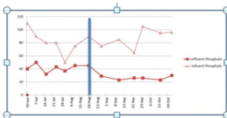
**Figure 6:** Soluble phosphate in the influent and effluent
