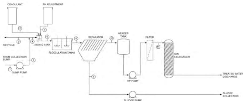
**Figure 1:** *Process flow diagram of original process configuration of the Casey WTP*
