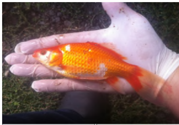
Figure 4: Goldfish after 5 months in primary effluent
