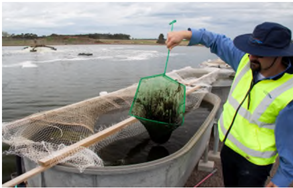
Figure 1: Control tank – No fish heavy sludge accumulation
