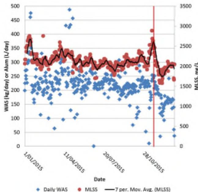
**Figure 4:** *Daily Measured MLSS and Calculated Volume of Sludge Wasted. Line Indicates Date of Implementation.*
