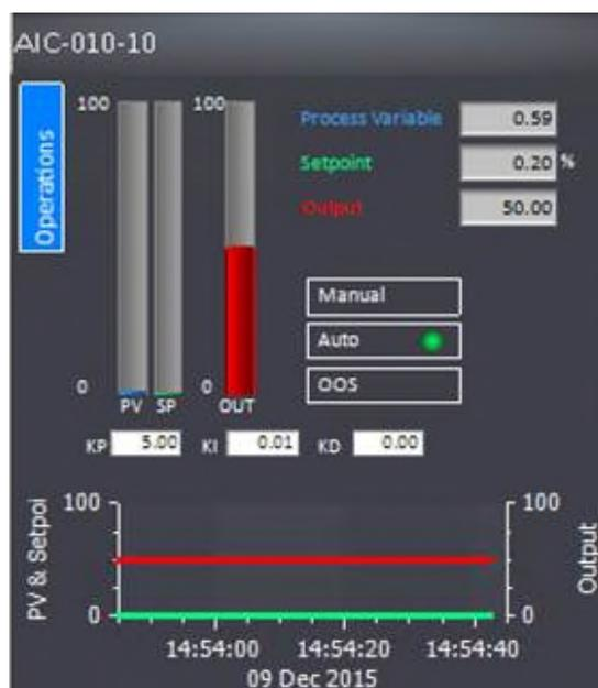
**Figure 1:** *Orthophosphate Trim Controller Faceplate (ClearSCADA).*
