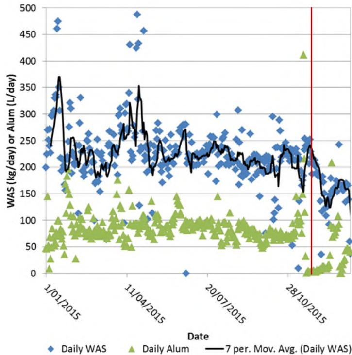
**Figure 3:** *Reduction in ACH Consumption and Volume of Sludge Wasted (Jan '15 to Jan '16). Line indicates Date of Implementation.*
