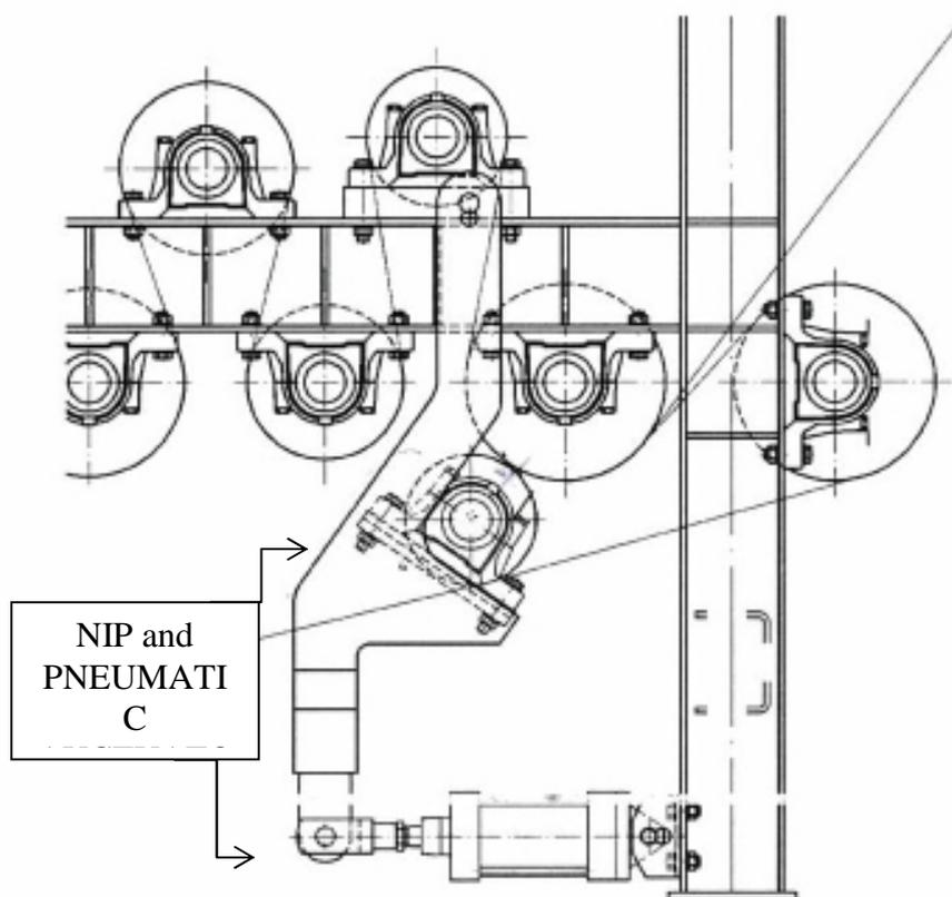
**Figure 1:** *Belt Filter Press Nip.*
