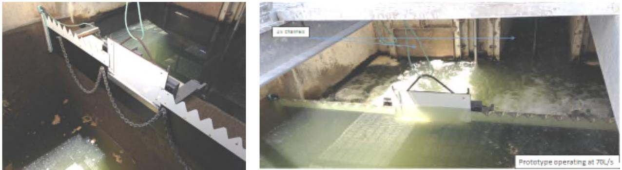
**Figure 2:** *Completed Prototype Weir.*
