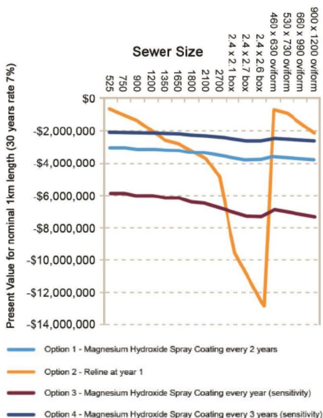
**Figure 3:** *Cost comparison MHL costing v/s plastic lining*
