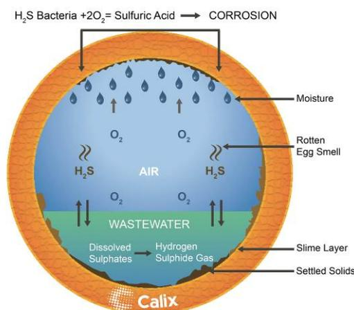
**Figure 1:** *Mechanism of  $\text{H}_2\text{SO}_4$  Production in Sewers*
