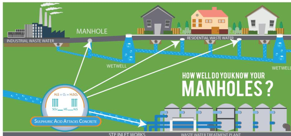
**Figure 8:** *Sewer Assets where Corrosion can Occur*
