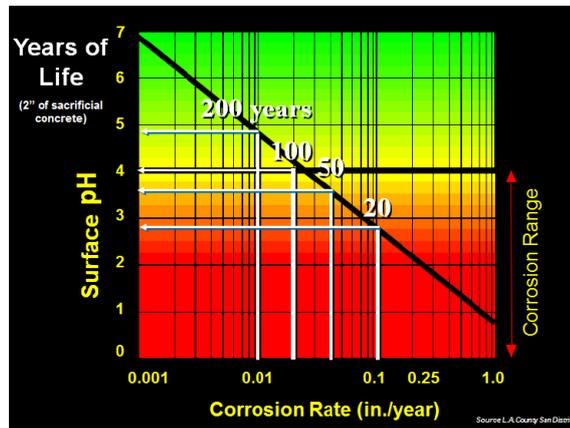
**Figure 5:** *Relation of Wall pH with Corrosion Rate and Life of Asset*
