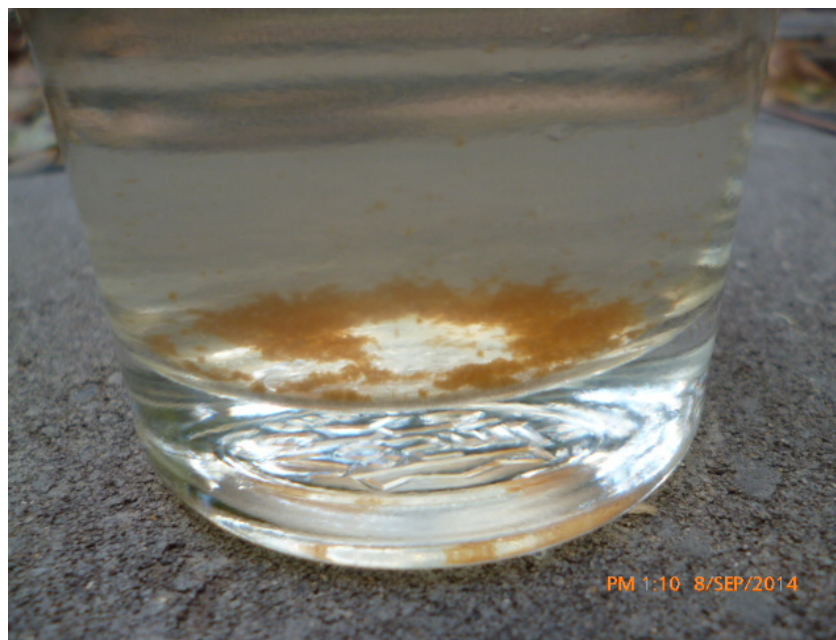
Figure 1: Oxidised Biofilm in Water Sample taken from a Customer's House
