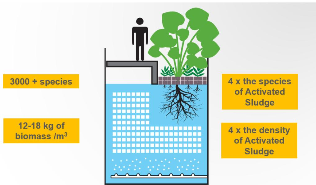
**Figure 1:** *Food Chain Reactor (FCR) – Cross Section of the Reactor Process*
