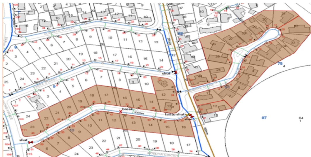
Figure 4: Consequences if DN100 valve failed to shut, 41 houses affected instead of 20
