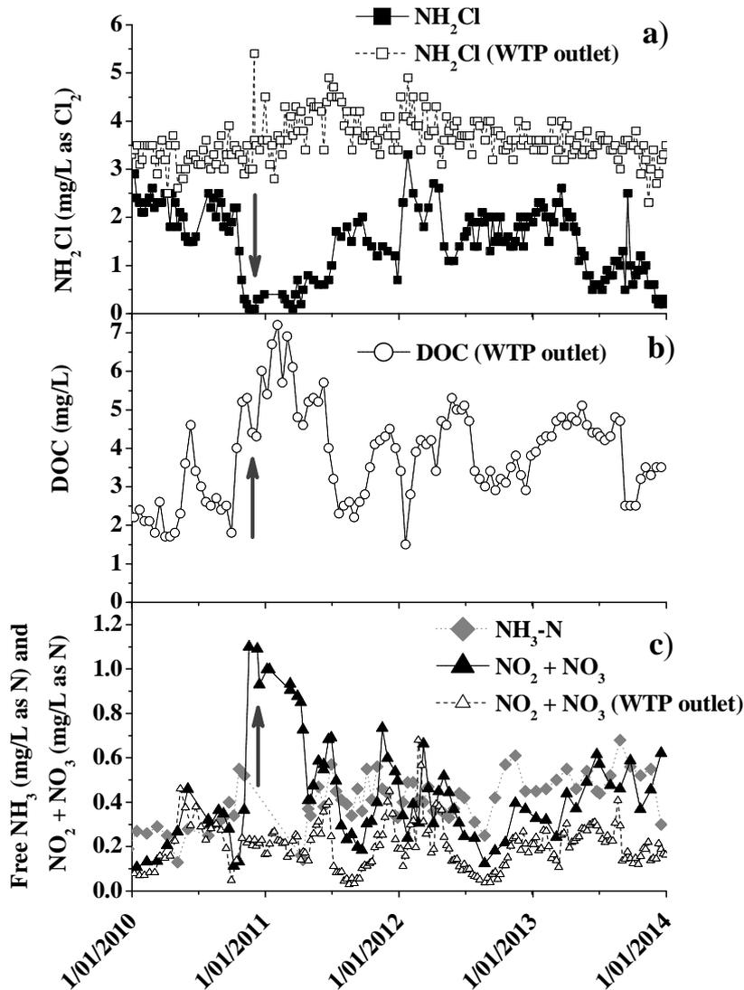
**Figure 2:** *Water quality at Raukkan Tank (full data points) and Tailm Bend WTP product water (open data points) a) monochloramine residual b) DOC concentration; and c) free ammonia and total oxidised nitrogen*
