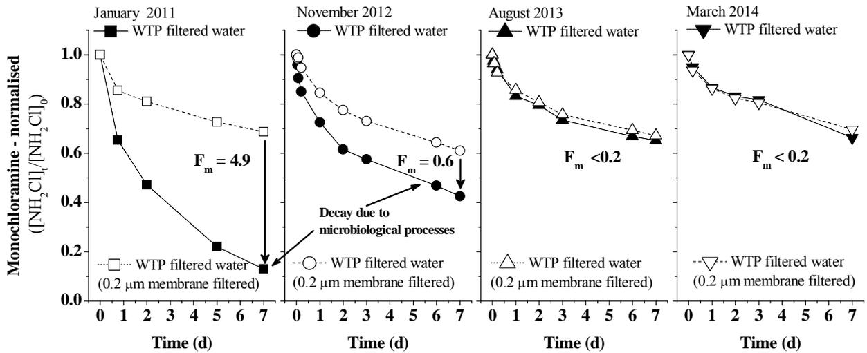
**Figure 4:** *Monochloramine decay in Tailem Bend WTP filtered water, with and without filtration through a 0.2 µm filter, January 2011 – March 2014*
