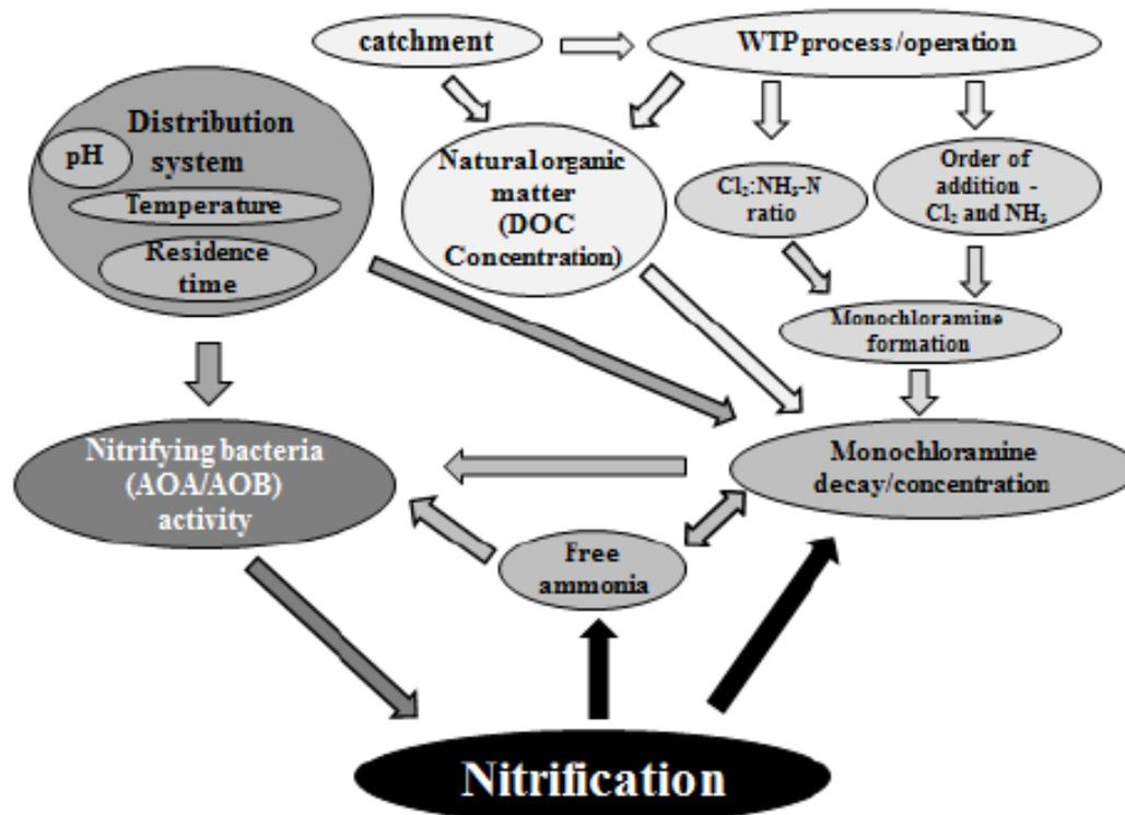
**Figure 1:** Factors that impact on monochloramine decay and nitrification
