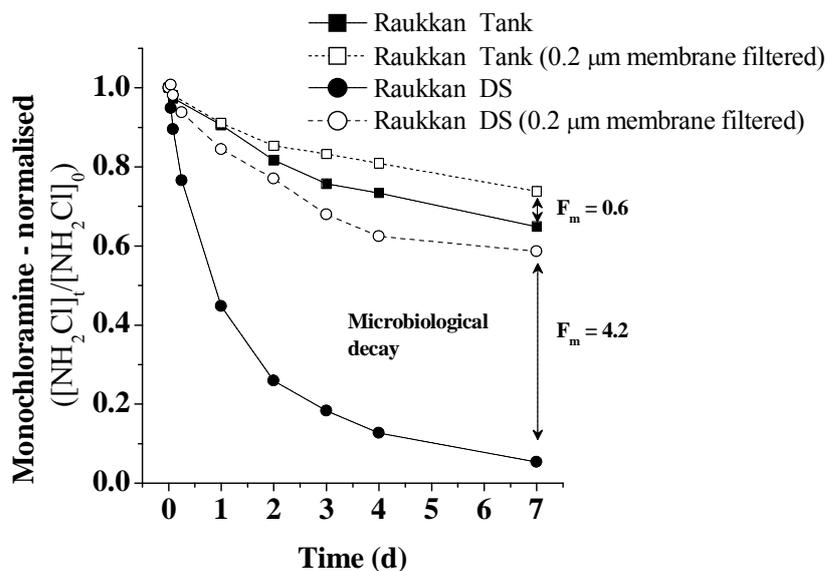
**Figure 5:** *Monochloramine decay in Raukkan Tank and distribution system*
