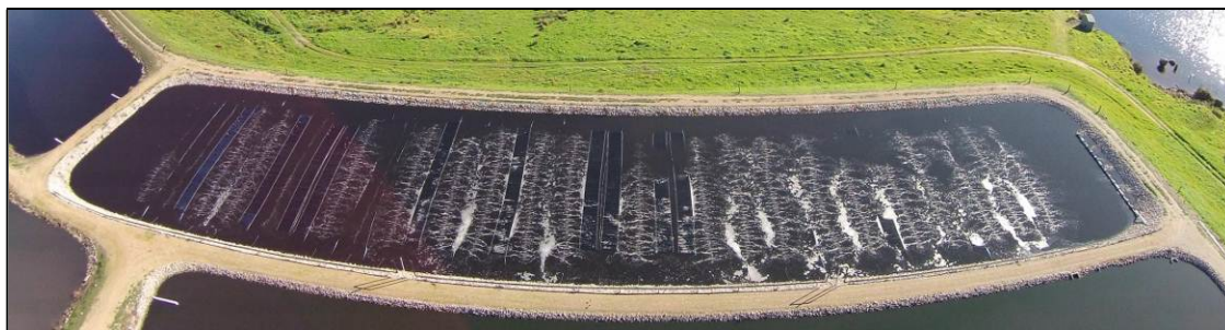
Figure 4: Photo taken by the drone of a wastewater lagoon showing diffuse aeration pattern.
