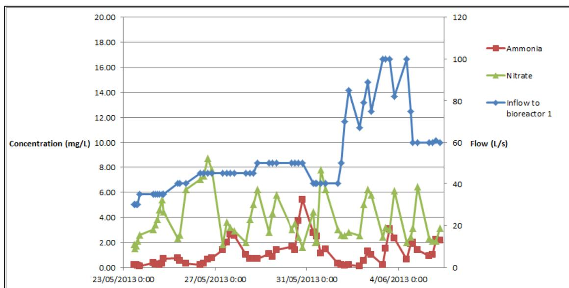
**Figure 6:** *Trend of nitrogen removal performance and bioreactor 1 inflow during outage*
