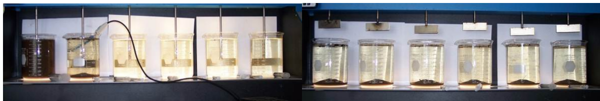
Figure 4: Jar tests on the Macalister River water Licola.
