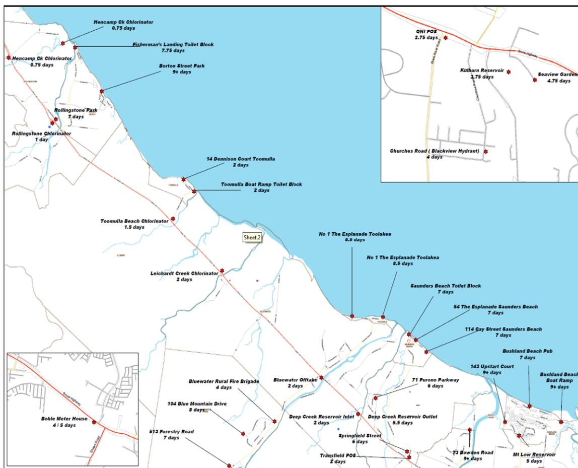
**Figure 1:** Schematic showing sample points and corresponding water age. (NWTP to Kulburn Reservoir =46.4km)
