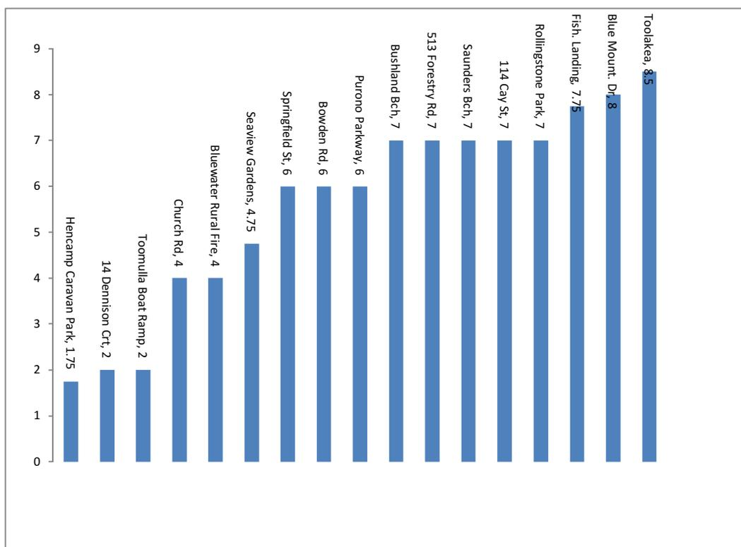
**Figure 3:** *Days taken for water to travel from NWTP to the reticulation sample points.*
