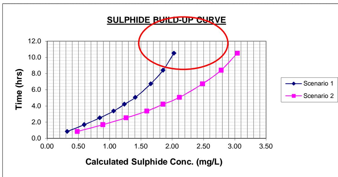
**Figure 1:** *Predicting sulphide concentration in a sewer*
