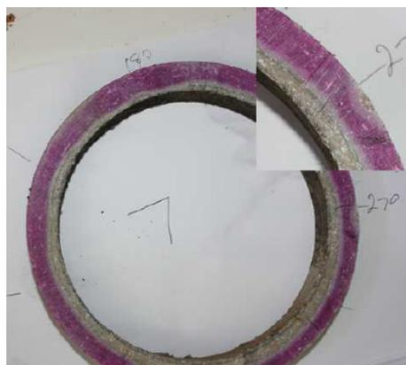
**Figure 6:** *AC Sewer rising main-internal leaching due to H<sub>2</sub>S gas*
