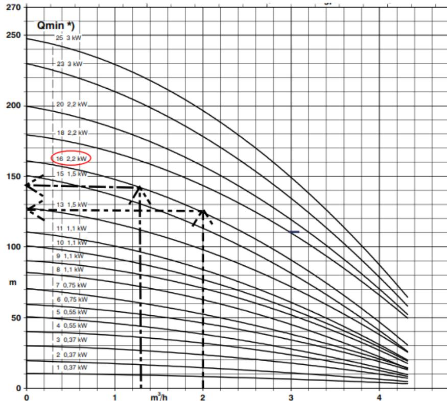
**Figure 2:** KSB Movitec V(S)2 curve (high pressure pump)
