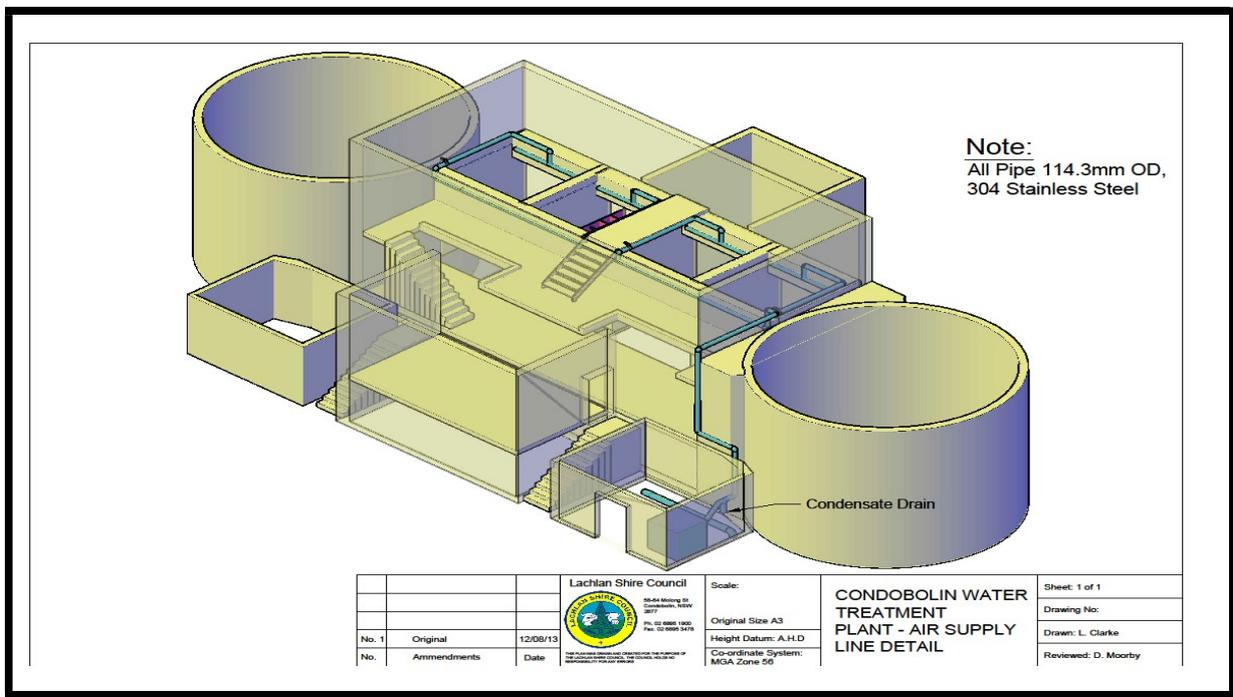
**Figure 5:** 3D General arrangement of Air Scour System
