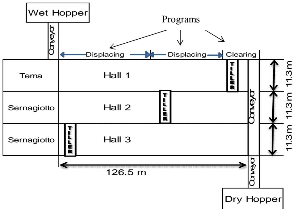
**Figure 1:** *Solar Drying Hall dimensions*
