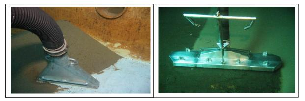
Many different types of suction hose have been tried (and discarded) as well – lifting weights have to be balanced with crushing and buoyancy issues. The average sized tank requires 40 to 60 meters of vacuum hose, with larger storages using 100 meters plus, so the equipment vehicles just kept on growing and growing over the years, along with the process knowledge.
