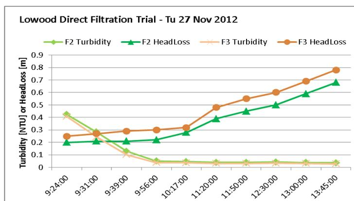
**Figure 1:** Graph showing filtered turbidity and head loss during DF trial
