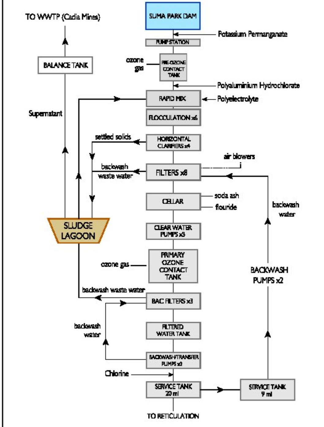
**Figure 1:** Process Diagram for Orange WTP
