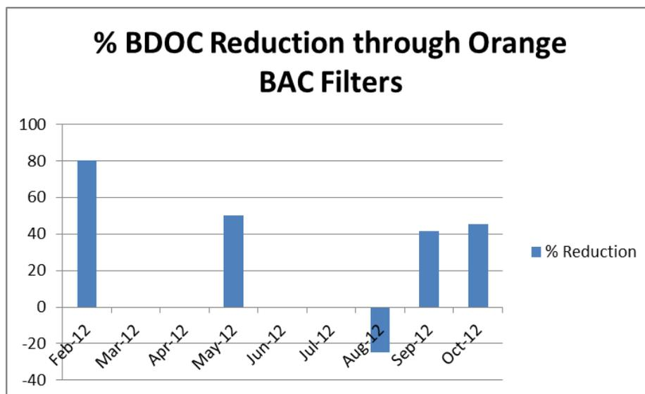
**Figure 3:** *BDOC Reduction for Orange WTP BAC Filters*
