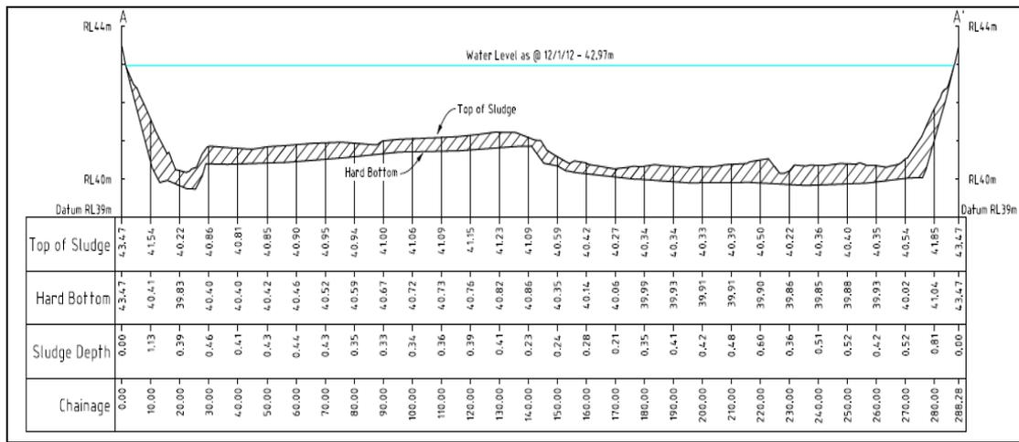
**Figure 5:** Longitudinal section view of deposition profiles
