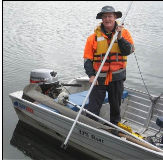
**Figure 3:** *Deploying GPS-integrated Infra-red sludge particle density detector*
