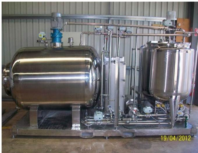
**Figure 1:** 500L Micro MHL Batching Plant with 2000L Storage
