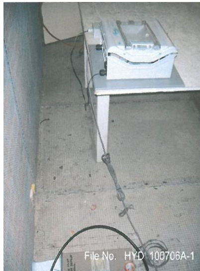
Figure 1: Mains terminals conducted disturbances test
