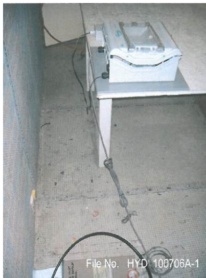
Figure 1: Mains terminals conducted disturbances test
