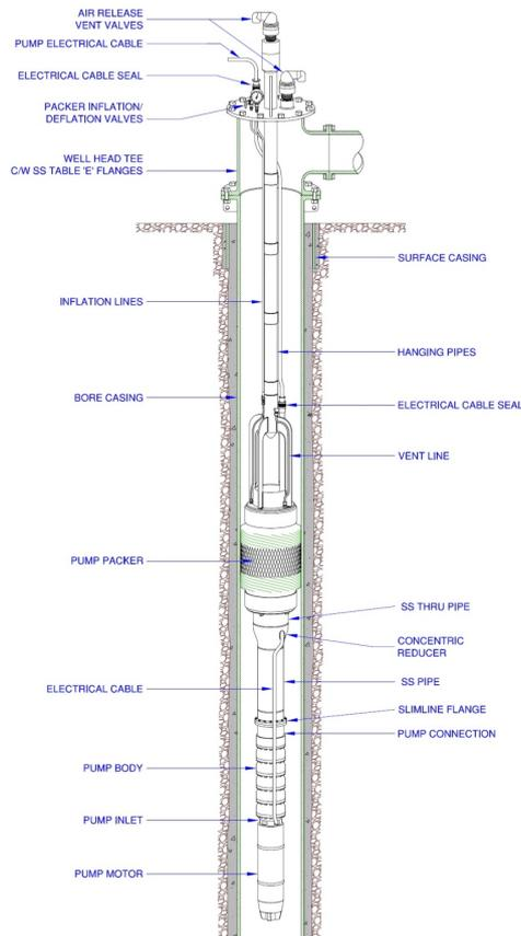
**Figure 1:** *Illustration of typical Riserless Pump Packer system (source: AGE Developments 2011)*
