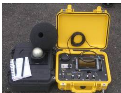
Figure 2: SmartBall with Foam Cover and Tracking Unit
