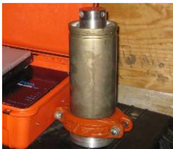
Figure 9: Acoustic Pulser used for Pipe Wall Assessment (PWA)
