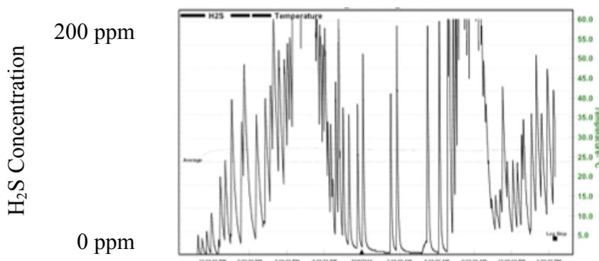
**Figure 3:** *H<sub>2</sub>S gas monitoring at the end of a rising main at Ayr – ProBac dosing*
