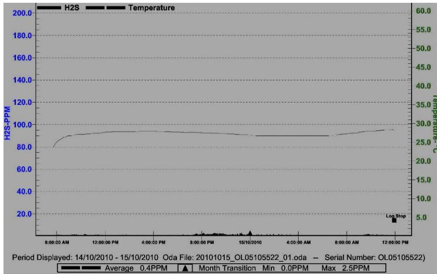
**Figure 5:** *H<sub>2</sub>S gas monitoring at the end of the SPS 5 rising main at Ayr – Biosol dosing. Average daily odour has been reduced to 0.4ppm and peak to 2.5ppm.*
