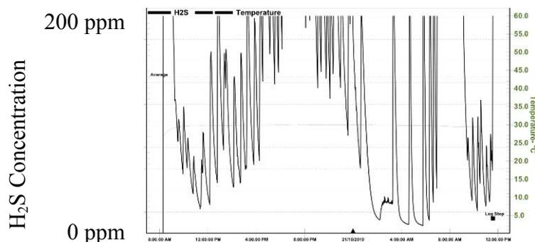
**Figure 2:** *H<sub>2</sub>S gas monitoring at the end of a rising main at Ayr*
