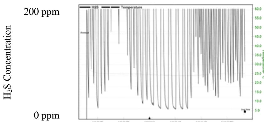
**Figure 4:** *H<sub>2</sub>S gas monitoring at the end of a rising main at Ayr – Actizime dosing*
