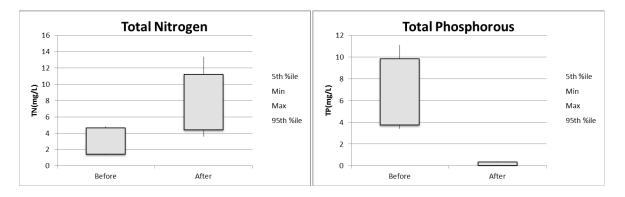
It can be seen that there has been a significant decrease in the total suspended solids, biological oxygen demmand and total phosphorous. This is because the membranes provide a physical barrier as opposed to gravity clarification, and also a more robust process for supplying aeration.
