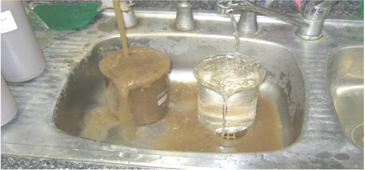
**Figure 2:**     *Raw water @ 4220ntu (left) and the final treated water @ 0.24ntu*
