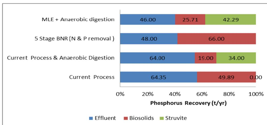
**Figure 2:** *Phosphorus stream compositions (From BioWin modelling)*
