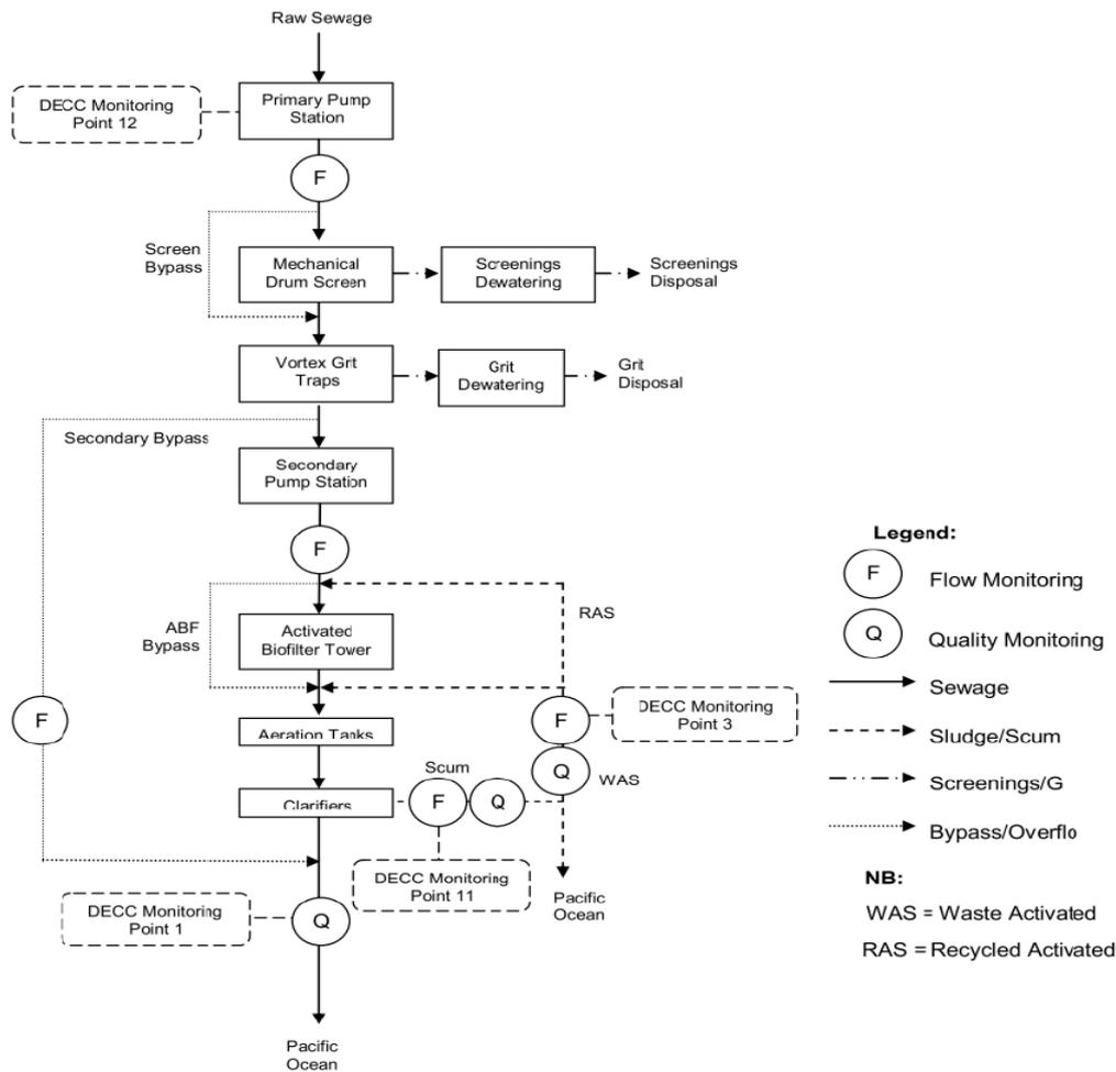
**Figure 1:** *Burwood Beach WWTW process flow diagram*
