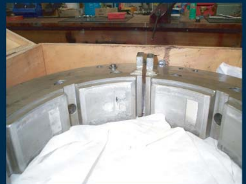
Vertical Pump Bearing Wear by the Pump Resonance
