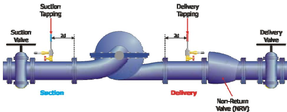
**Figure 5:** *Typical Tapping Arrangement*
