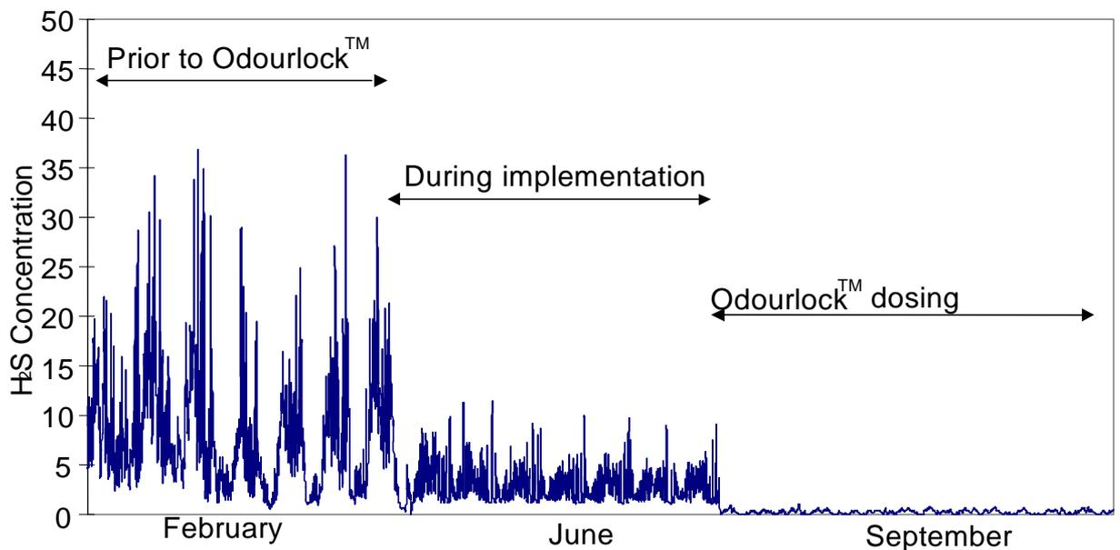
The reduction in sulphide levels corresponded with a decrease in the number of odour complaints received by the water board by 50% thus demonstrating to their ratepayers and the NSW EPA that they have tackled the sewage odour problem successfully. Further, reduced H<sub>2</sub>S<sub>(g)</sub> levels within the network minimises corrosion of valuable sewerage infrastructure.
