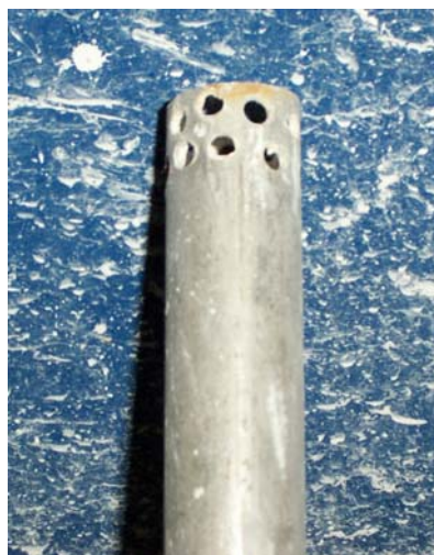
Figure 4: Lime System Suction Tube Prior to Modifications. Hole Diameter = 3mm
