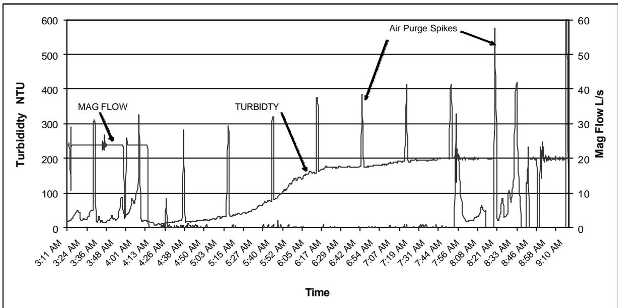
Figure 4 shows the spikes due to the air purge and also the increase in the turbidity reading during the plant shut down.
