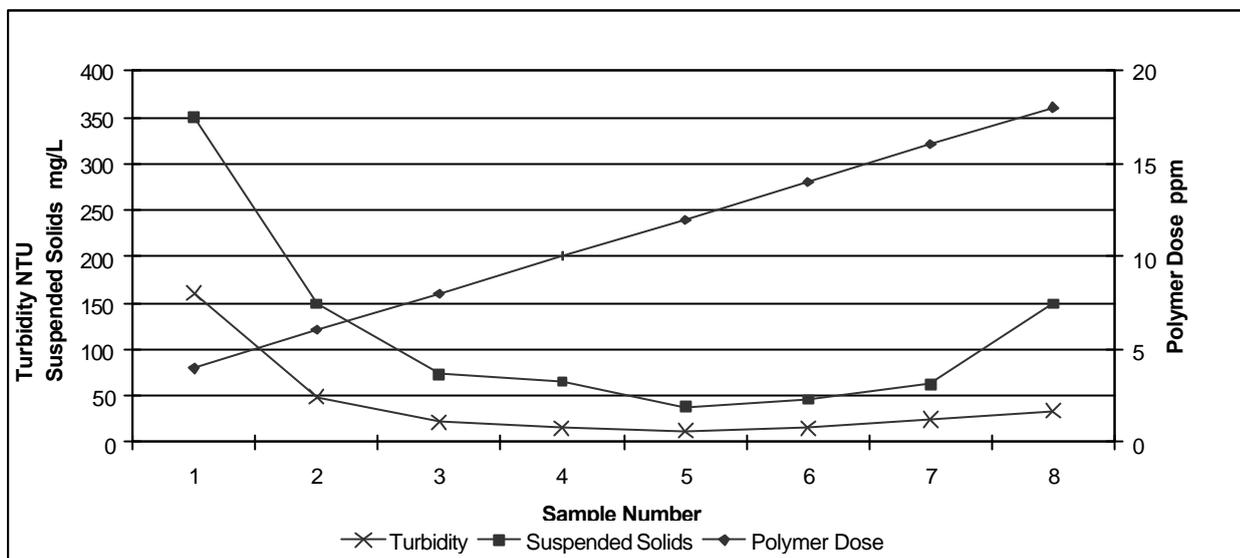
Figure 5 shows that it is possible to automate the dosing rate to obtain the lowest turbidity.
