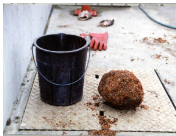
Figure 5: Mud ball found in a filter that had completely failed at Traralgon
