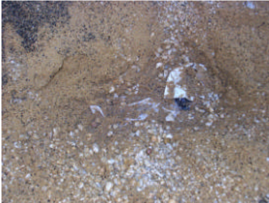
Figure 9: Support gravel has been completely displaced. A still area in the air scour pattern was the first indication
