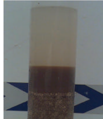
Figure 7: An example of a shake test. Layers of media, sludge and water can clearly be seen
