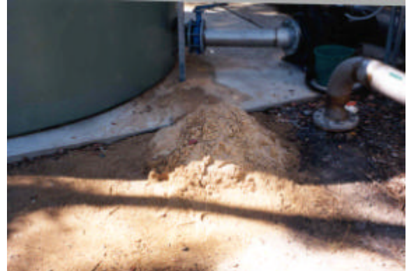
Figure 10: Result of a broken under drain nozzle. Sand entered the backwash tank and was redistributed to other filters. This required significant work to remove the sand and resulted in other filter rebuilds.
