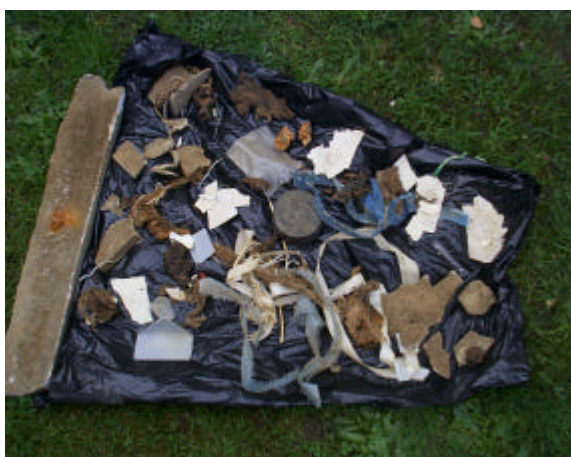
Figure 4: Rubbish removed from within the filter during refurbishment at Morwell
