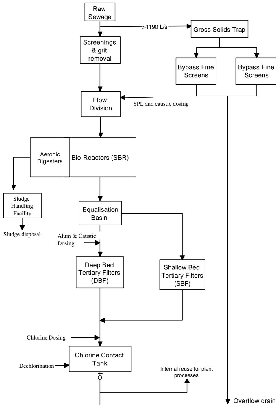
The SBRs at Winmalee STP were designed for biological and chemical phosphorus removal by the addition of alum at a concentration of 6 – 8 mgAl/L. An optimisation programme was carried out since September to enhance the phosphorus removal in the SBRs process by replacing alum with SPL (Ferrous solution) which is a by-product of steel manufacture at 160 g/L of Iron.
