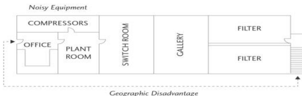
It would appear little thought has been given to the distances and pathways an Operator needs to travel when collecting samples or inspecting the various components of the plant. eg. The door to
