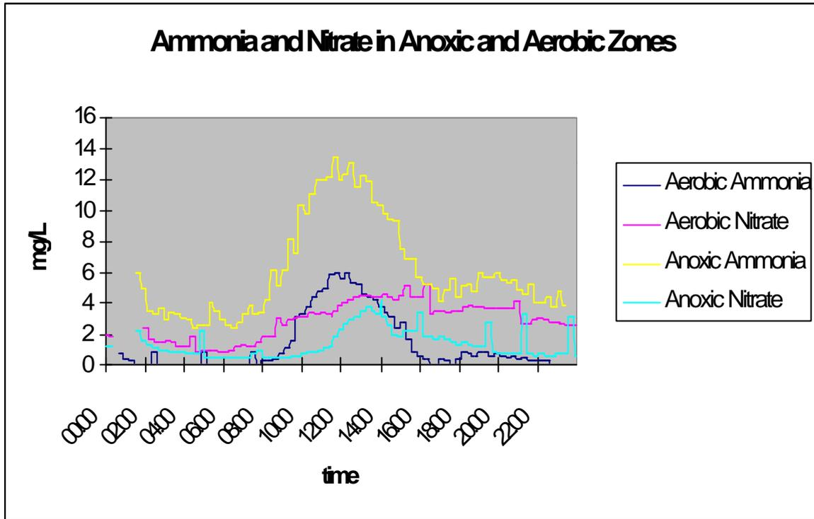
Discharge ammonia and nitrate levels on a daily average basis are around 1 mg/L and 2.5 mg/L respectively. DO levels are maintained at a constant setpoint at all times.
