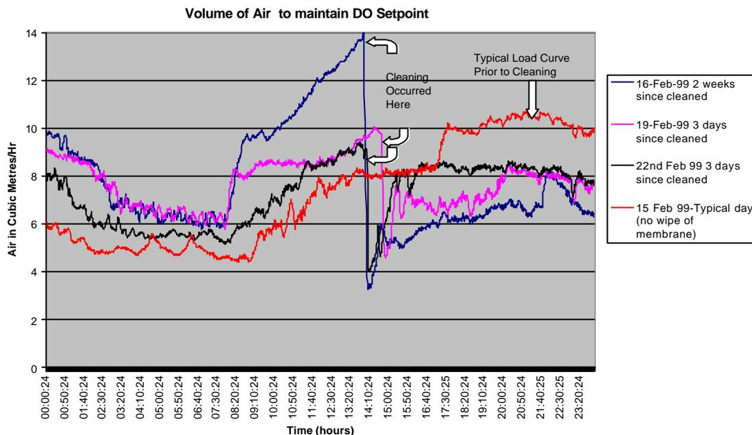
The above graph shows the considerable error which can occur within hours let alone days of cleaning and recalibrating. An appropriate control strategy to achieve the biological conditions you want at each and every loading condition the plant sees can only be determined with accurate data on DO levels.
