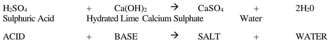
The salts produced can in some cases often protect the rest of the structure from further degradation, however this is dependent upon various factors including the nature of the effluent and flow characteristics of the system.
