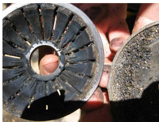
Figure 3: Deposits under nozzle cap
