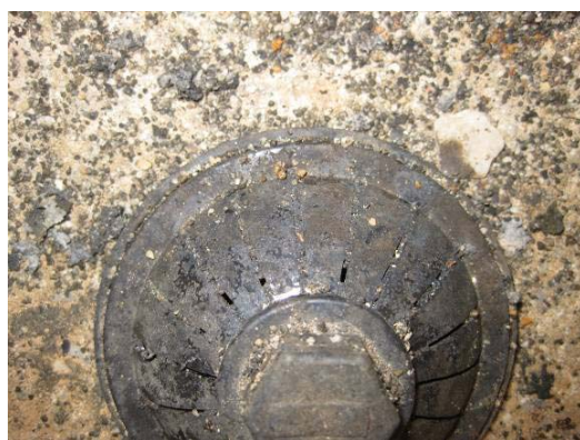
Figure 2: Nozzle slot blockage
