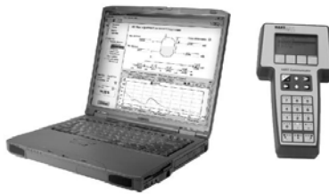
Figure 4: Notebook PC and HART communicator, typical programming tools
