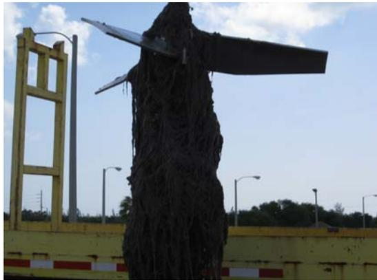
**Figure 1:** *Fouled impeller*
