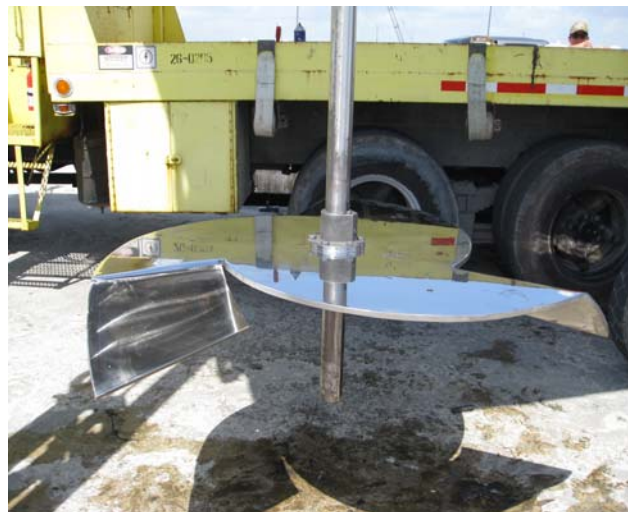
Figure 3: New swept-back blade and angled tip that produces an axial flow
