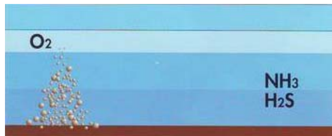
Figure 1: Ammonia and hydrogen sulphide generation from sediment/sludge
