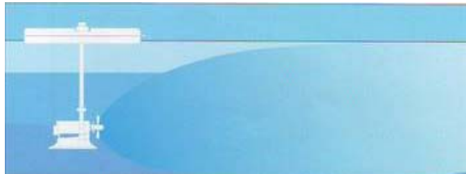
Figure 3: Artificial destratification introduced (mechanical circulation)
