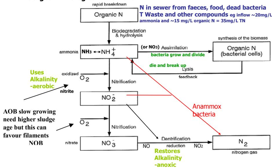
The above flowchart shows key chemical transformations carried out by nitrifying and denitrifying bacteria in BNR. The currently experimental ANAMMOX process provides a route for N removal using another group of slow growing bacteria that can change  $\text{NH}_3$  and  $\text{NO}_2$  into  $\text{N}_2$  gas without aeration.
