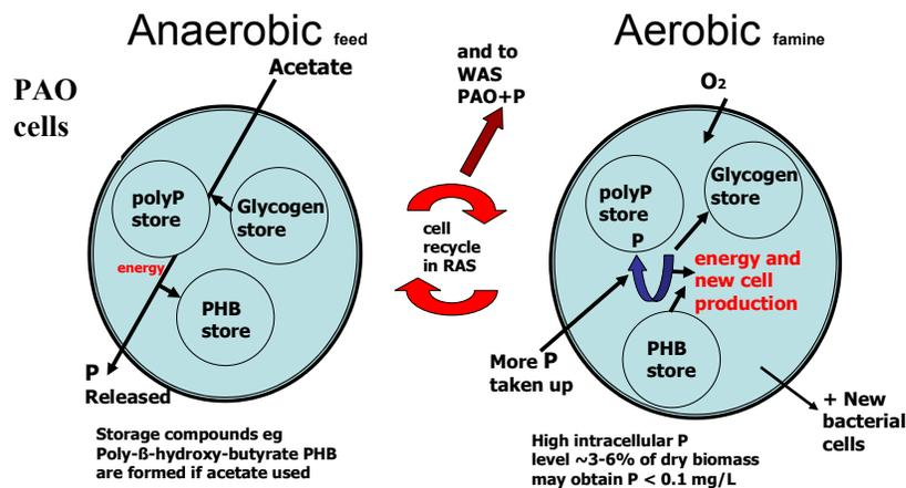
**PAO cycling** between aerobic and anaerobic conditions, taking up extra P (luxury uptake)
