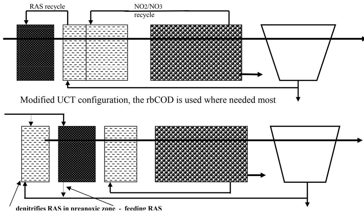
Modified Johannesburg configuration, increases size of anoxic sludge fraction
