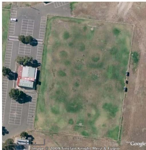
**Figure 3:** *Doughnut effect due to low supply pressure.*
