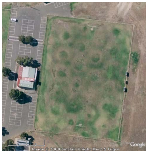
Figure 3: Doughnut effect due to low supply pressure.
